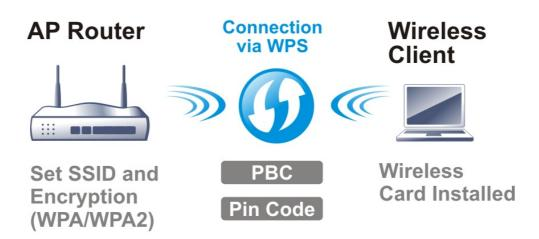
It is the simplest way to build connection between wireless network clients and VigorAP 1000C. Users do not need to select any encryption mode and type any long encryption passphrase to setup a wireless client every time. He/she only needs to press a button on wireless client, and WPS will connect for client and VigorAP 1000C automatically.
