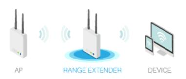
The access point can act as a wireless repeater; it can be Station and AP at the same time. It can use Station function to connect to a root AP and use AP function to serve all wireless stations within its coverage.
