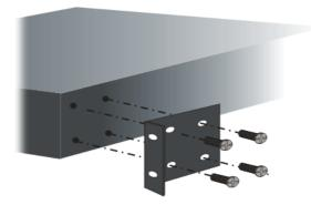
2. Then, install the VigorSwitch (with rack mount kit) on the 19-inch chassis by using other four screws.
