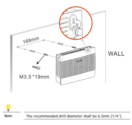
4. When you finished about procedure, the router has been mounted on the wall firmly.
