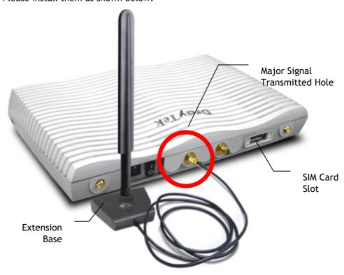
Note, if only one antenna shall be installed, please use the mounting hole (major signal transmitted hole) near to the SIM card slot.
