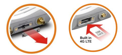
There are two types of antennas provided for Vigor2866Lac, which must be installed in different locations carefully and correctly. Wrong installation might cause bad signal of wireless connection. Therefore, pay attention to the installation of antennas by referring to the following illustration.
