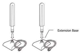
There are two mounting holes for installing antennas with extension base on Vigor router. Please install them as shown below.
